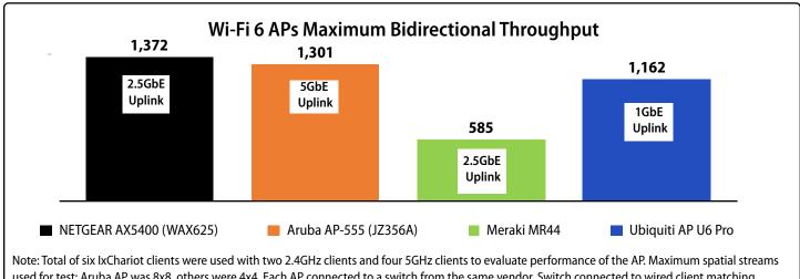
Note: Total of six IxChariot clients were used with two 2.4GHz clients and four 5GHz clients to evaluate performance of the AP. Maximum spatial streams used for test: Aruba AP was 8x8, others were 4x4. Each AP connected to a switch from the same vendor. Switch connected to wired client matching uplink speed.
